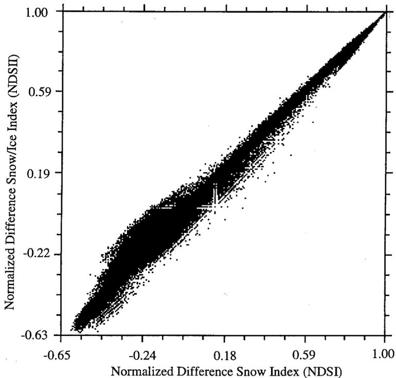
Figure 5. Comparison between the NDSI and the  $\text{NDSII}_{\text{TM}}$ , as calculated from a Landsat TM image acquired on 16 August 1996, for 160 000 pixels from a 400 by 400 pixel subset image centred at  $101^{\circ}30'E$  and  $37^{\circ}42'N$ . This subregion contains the snow/ice area shown in north-western part of figure 4.
