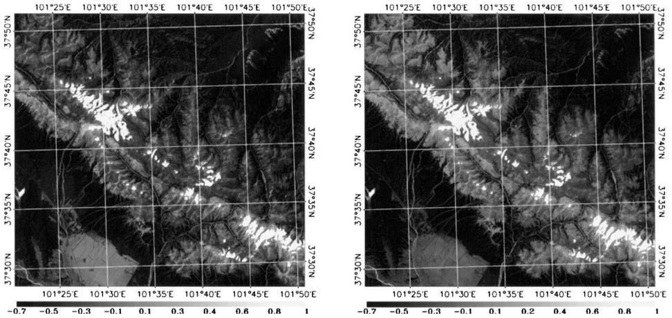
Figure 4. Spatial distributions of (a) the NDSI and (b) the  $\text{NDSII}_{\text{TM}}$ , as calculated from a Landsat TM image acquired on 16 August 1996.
